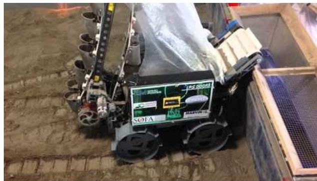
Figure 3: The robot created by the sixth year team. This robot had a bucket ladder to mine regolith and a cleated belt for depositing it into the hopper.
