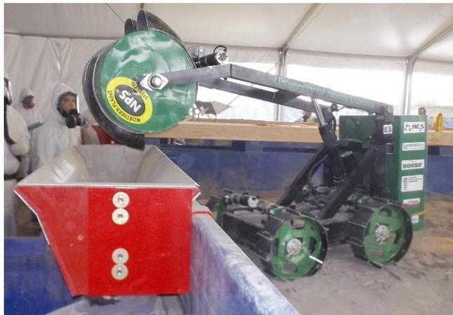
Figure 2: The robot used in the fourth year of the competition. This robot featured a spinning bucket with a baffle system.
