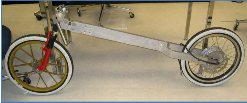
Figure 3 Frame, wheels and motor assembled
