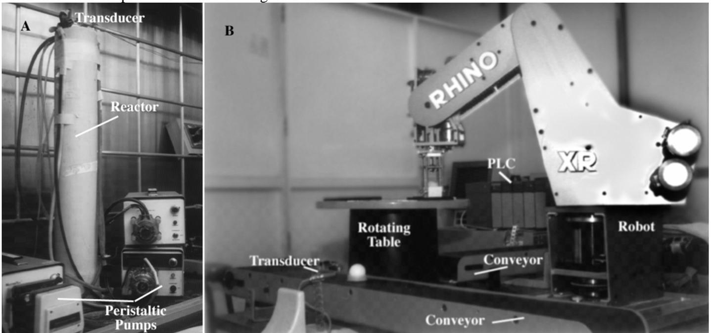
Figure 2. Experimental layout. Left (A), bacteria production cycle practical for PLC timers applications and right (B), a small production line for PLC counter applications learning.
