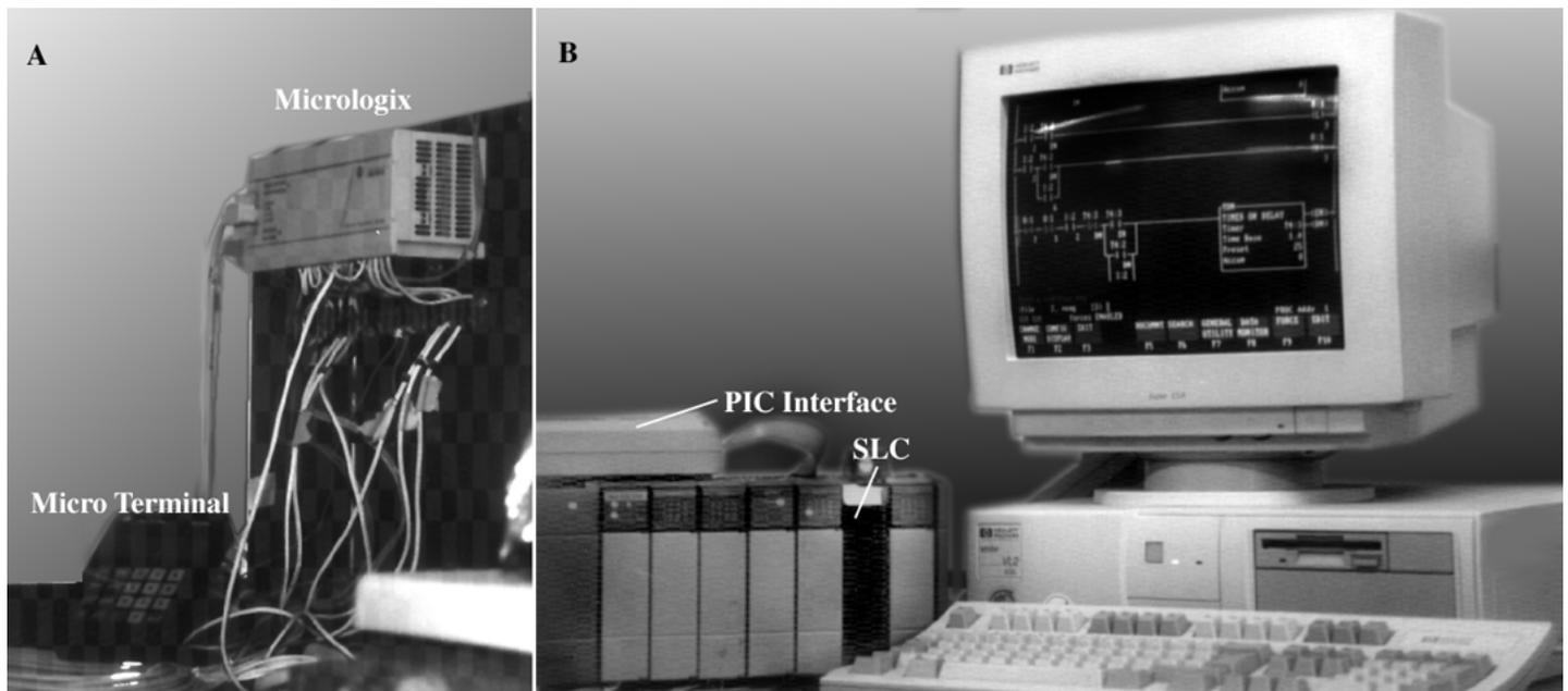
Figure 1. Workstation layout. (A) shows an arrangement with a Micrologix and the microterminal for programming, (B) shows a PC computer with a SLC interfaced through RS-485 (PIC).
