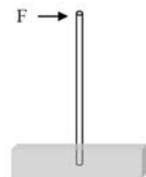
Here,  $k$  represents the stiffness of the pole and is measured in units of either N/m or lb<sub>f</sub>/ft.
