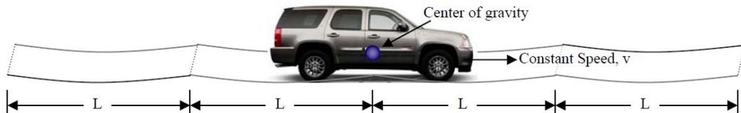
It takes  $(L/v)$  seconds to travel a distance  $L$  at a speed  $v$  (recall: distance = rate \* time). Then, the vehicle hits a “ridge” in the road at a frequency of  $(v/L)$ . At some speed,  $v$ , this frequency can excite the vehicle so that it bounces up and down. Thus, the roadway acts as a forcing.
