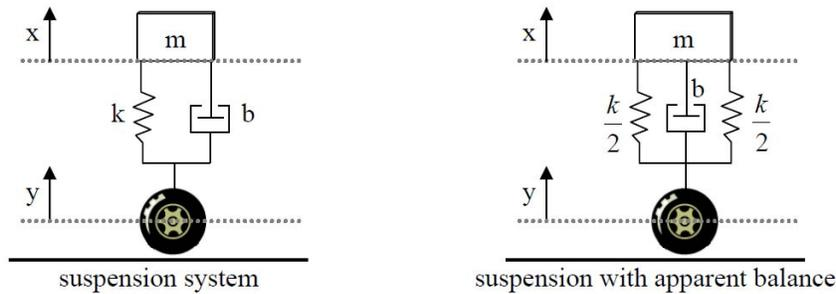
The schematic of the model for the oscillating pole, when damped is accounted for, is shown at right. Here, too, the stiffness could and sometimes is split into two springs, one on either side of the damper.
