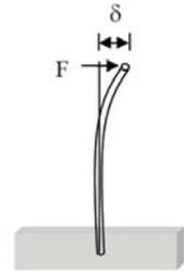
Now, the inertia of the system for the fundamental mode of vibration is modeled as a lumped mass that moves in only one direction (up and down for the car and side to side for the pole).
