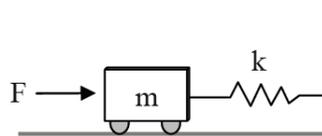
where  $F$  is the force causing the displacement. The wheels are assumed to have frictionless bearings and roll without slip.
