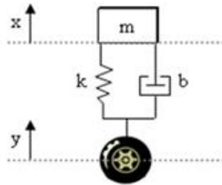
Figure 1: Single degree of freedom model of a car
