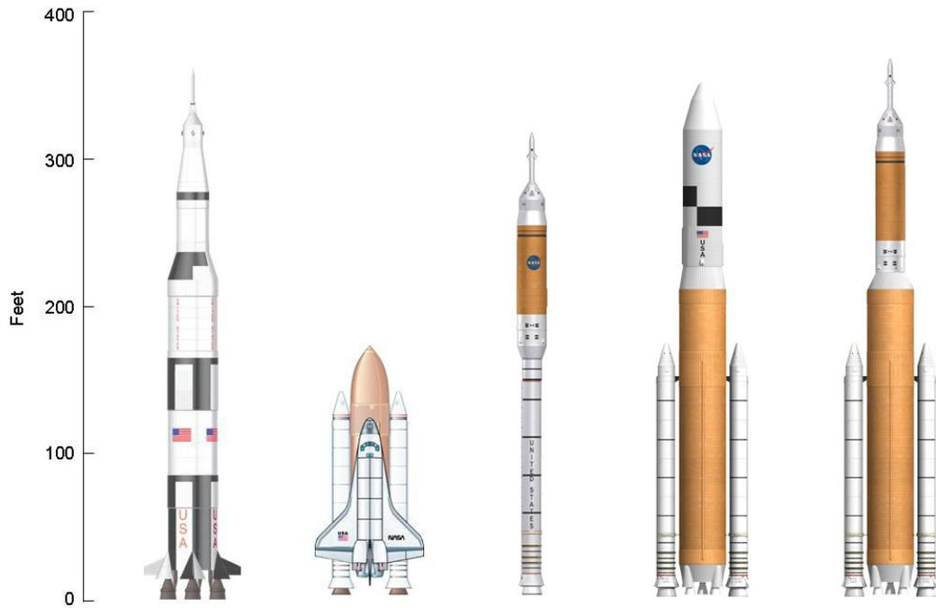
Figure 2: NASA rockets: Saturn V, Space shuttle, Ares I, Ares V, Ares IV
