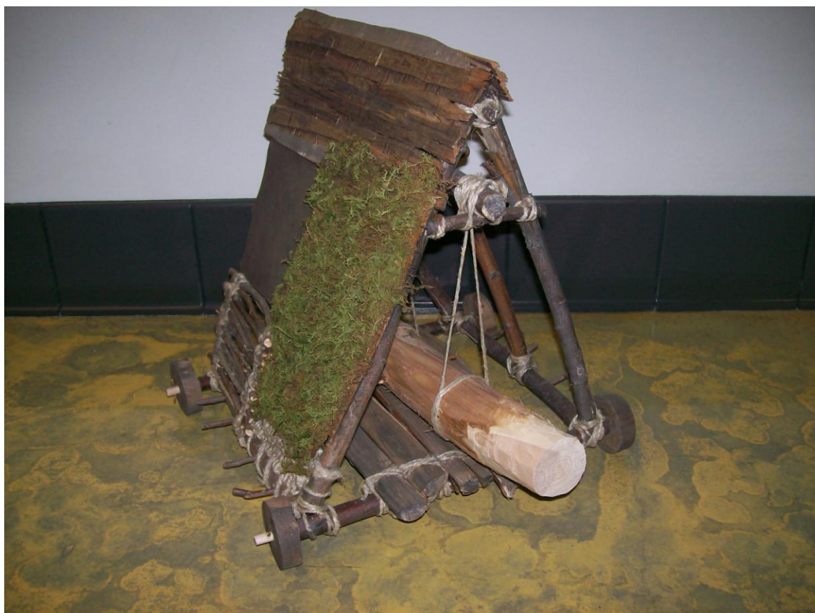
Figure 2. Scale Model of a Battering Ram with Protective Cover.
