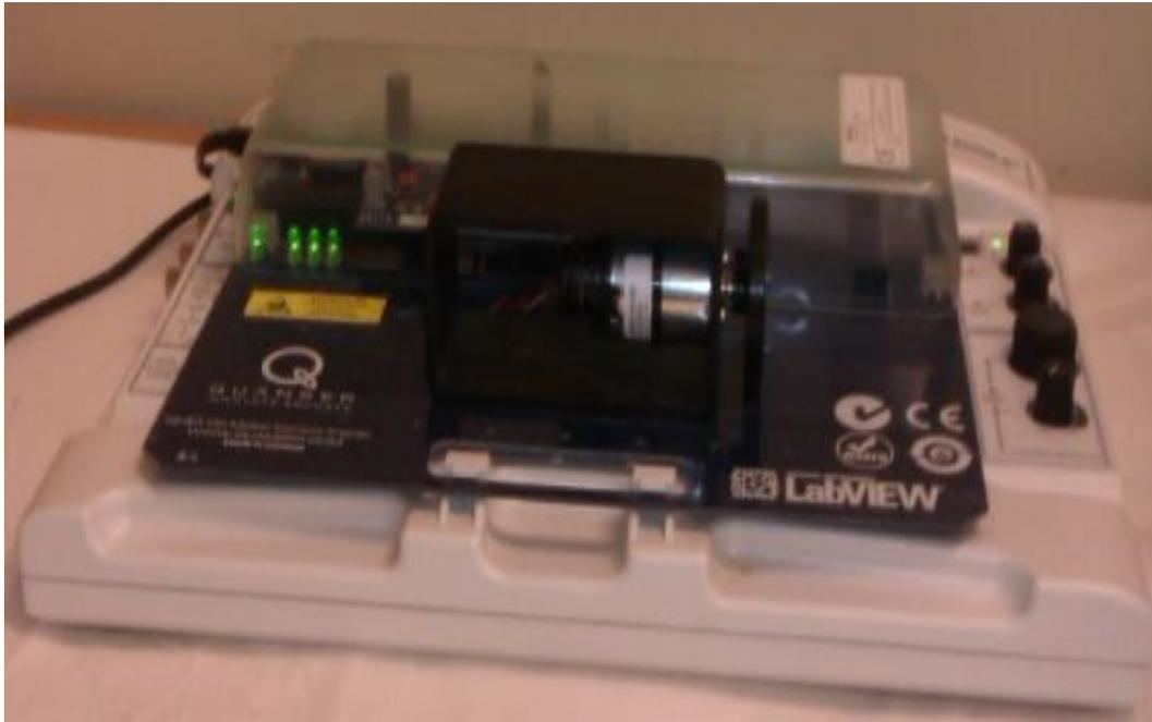
Figure 2. QNET™ DC Motor Control Trainer.
