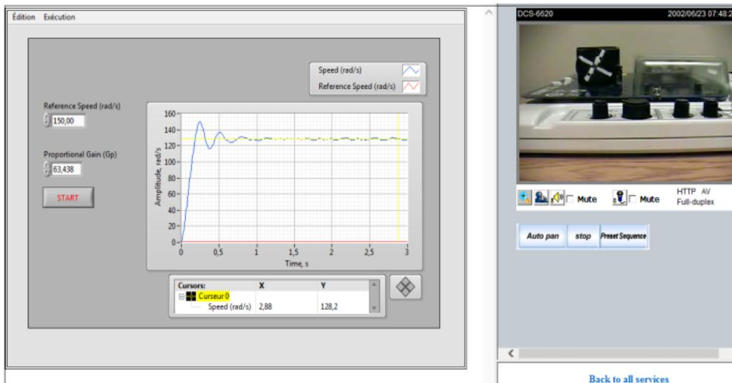
Figure 7. Interface of the closed loop with P Controller service.
