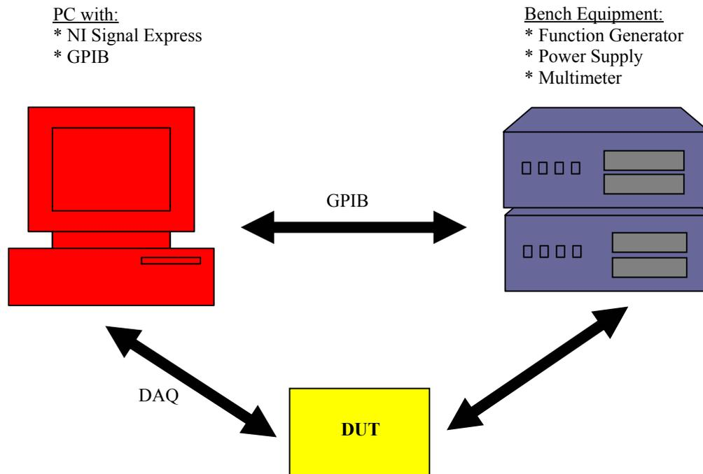
Figure 1 – Block diagram of the Signal Express test environment.
