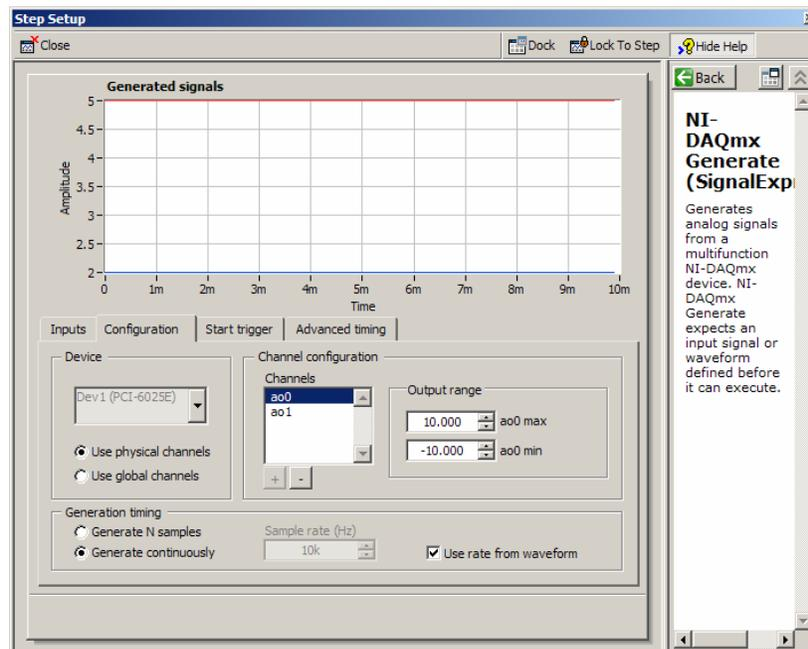
Figure 6 - Signal Express, Step Configuration
