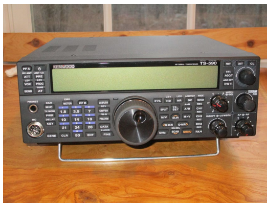
Figure 3. Receiver used for reception of HF signals.
