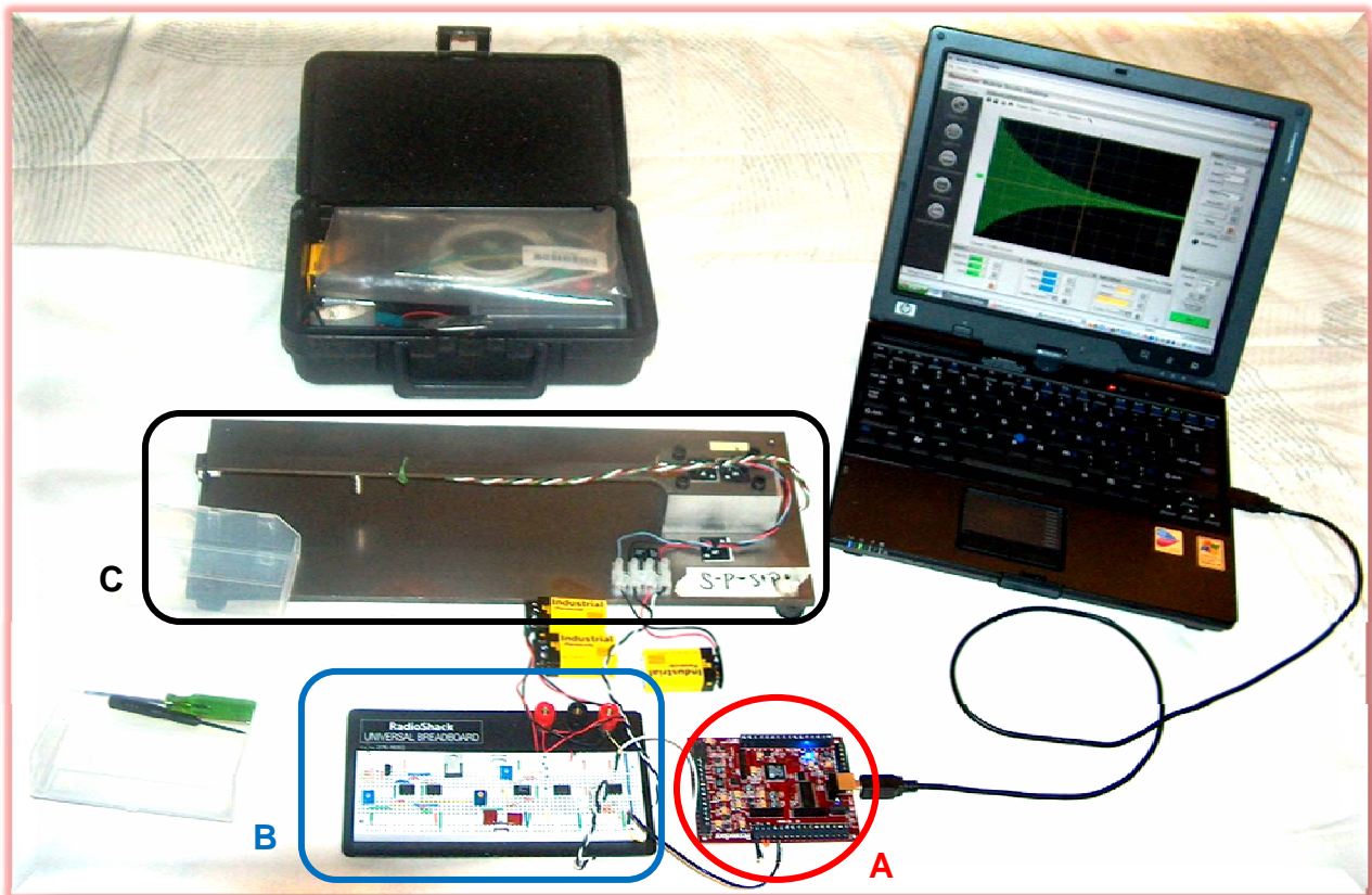
Example of Mobile Studio Experimental Setup for a Cantilever Beam with strain gauges mounted on the top and bottom of the beam: (A) Mobile Studio Board, (B) Interface Circuitry for (C) The Device Under Test. Not labels are the tool and parts kits, the laptop computer, DC power (9V batteries) and the USB cable.
