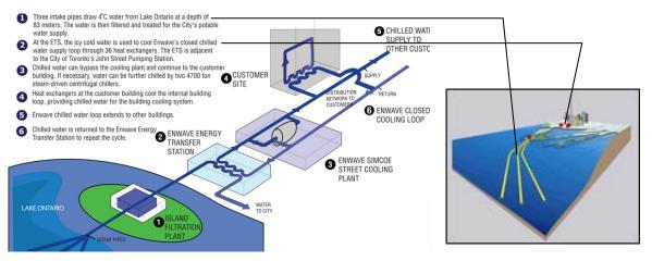
Figure 1. Deep Lake Water Cooling System Schematic [1, 2].
