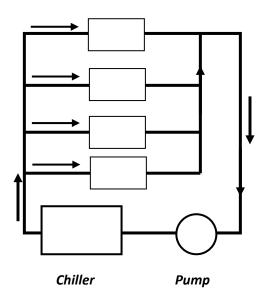
Figure E2. Z-layout schematic.
