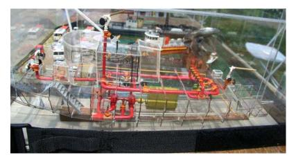
Figure 6. Cutaway Showing Piping for a Typical Fireboat [17].
