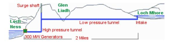
Figure 2. Schematic of FPHF [9, 10].
