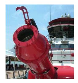
Figure 5. Fireboat Three-Forty-Three Primary Monitor (Nozzle) [14, 15, 19].
