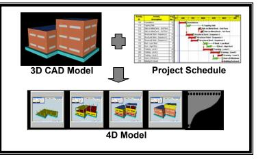
Figure 1: 4D CAD Model Development
