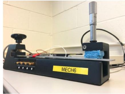
Figure 2. A cantilever beam with strain gauge
