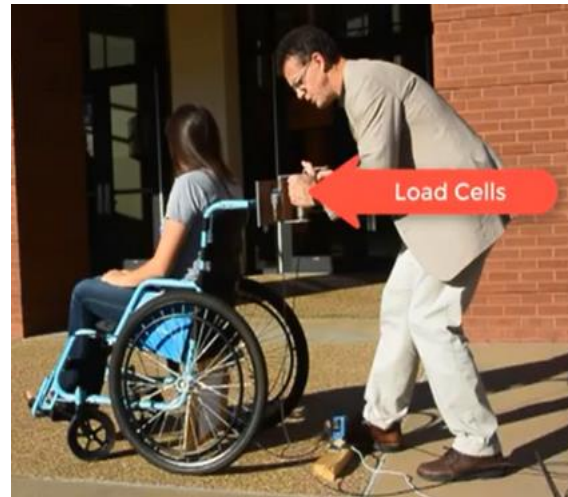
Figure 2. Impulse momentum module.
