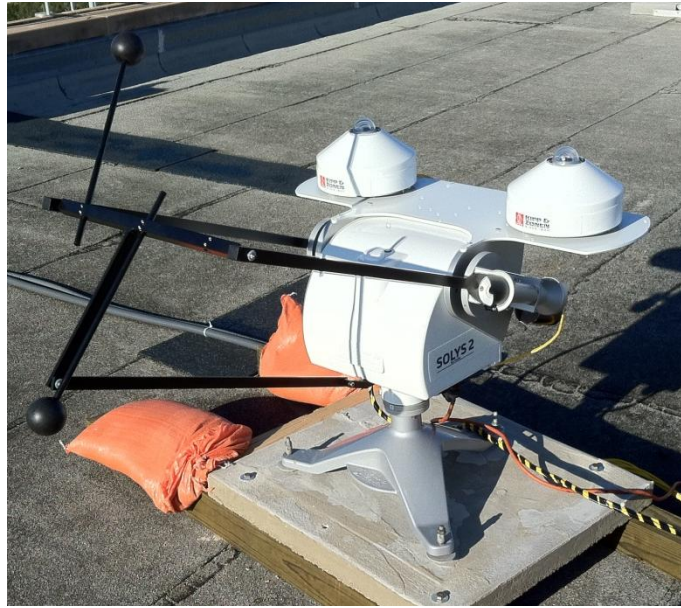
Figure 3 – This photo displays two pyranometers, one pyr heliometer, and the tracker.
