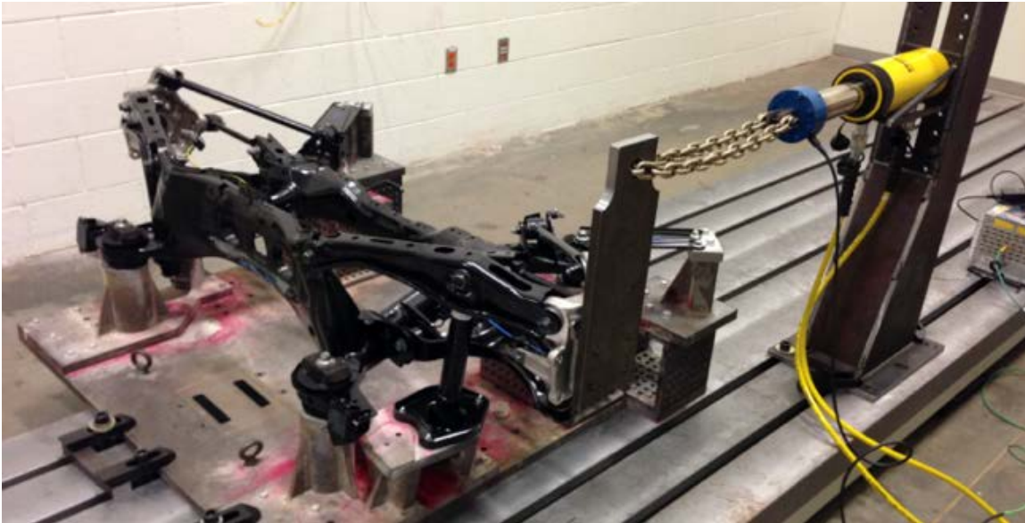
Figure 2. University laboratory replication of OEM structural test setup
