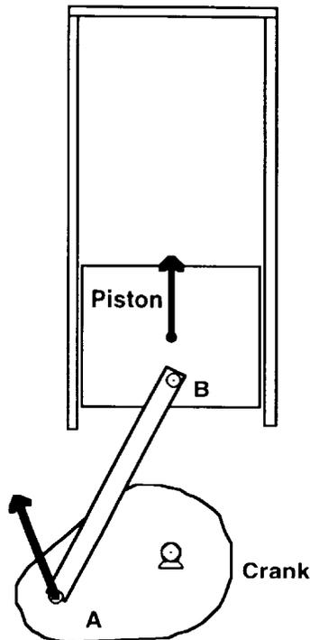
**Figure 3 Slider-crank mechanism**
