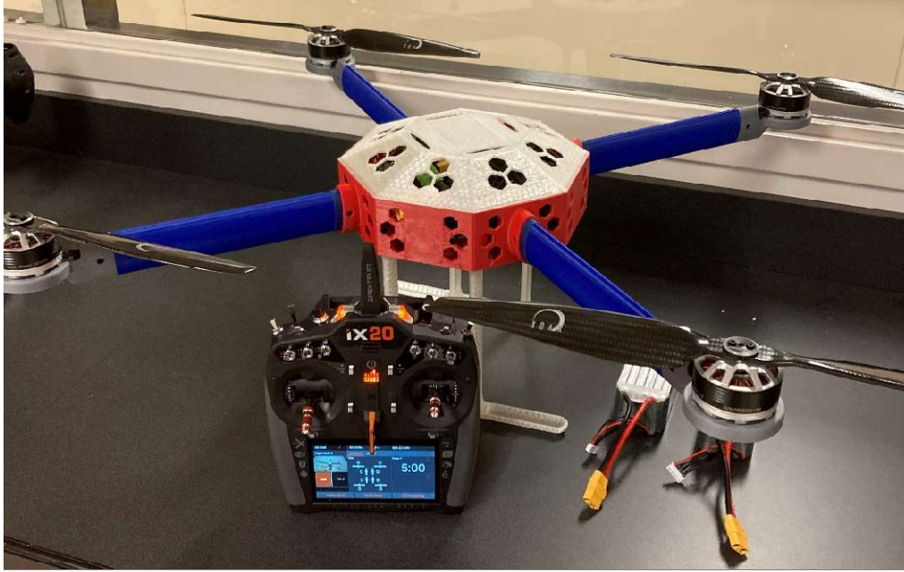
Figure 6: 3D Printed Assembly of the UAS
