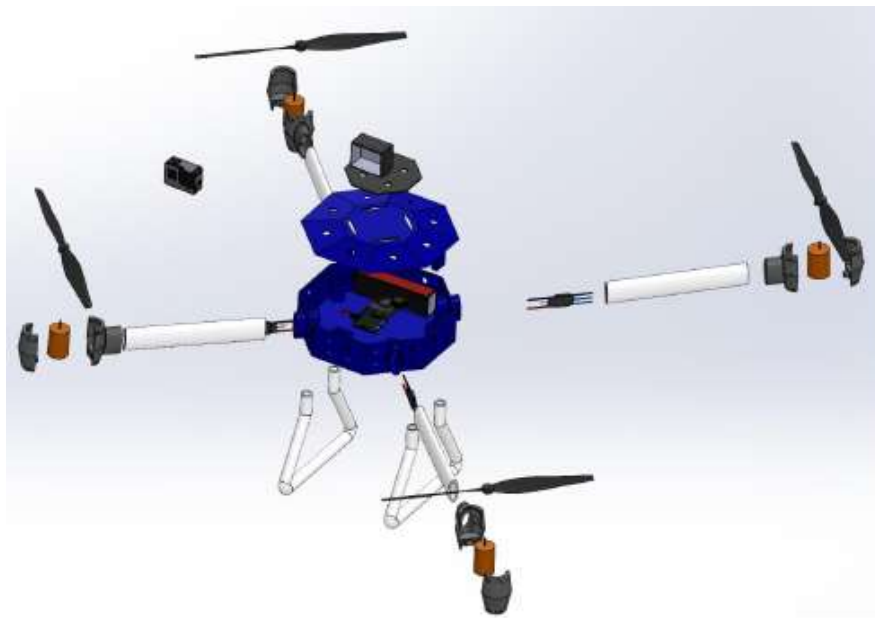
Figure 1: CAD Model of the Proposed UAS Design
