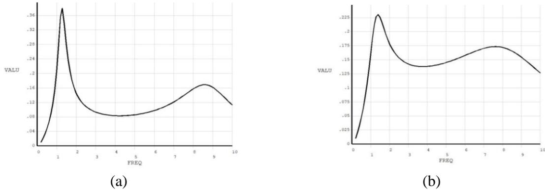
Figure 2 Responses of the sprung mass to harmonic excitations in the frequency domain. (a)  $C_s=1500\text{Ns/m}$  and (b)  $C_s=3000\text{Ns/m}$
