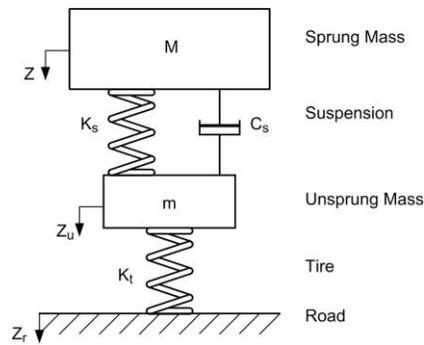
Figure 1. Schematic diagram of quarter-car model.  $M=450\text{Kg}$ ,  $m=90\text{kg}$ ,  $K_t=250000\text{N/m}$ ,  $k_s=31250\text{ N/m}$ , and  $C_s=3000$  or  $1500\text{ Ns/m}$ .
