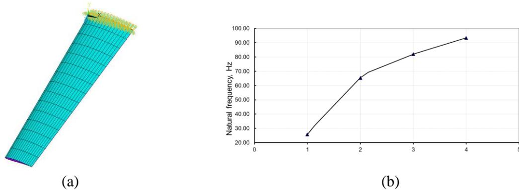
Figure 4. (a) Wing FEA model with rigid constraints applied at the root end, and (b) first four natural frequencies of the wing obtained from modal analysis.
