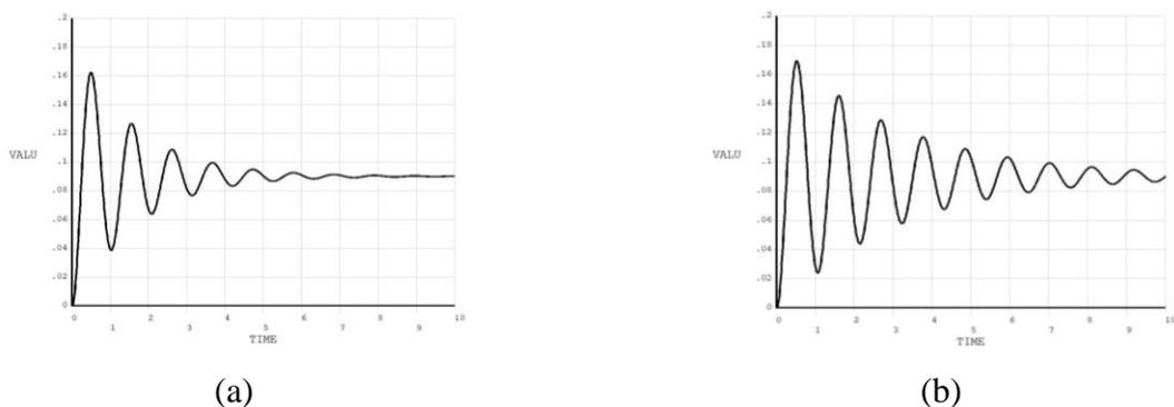
Figure 3. Responses of the sprung mass to impulsive excitations in the time domain. (a)  $C_s=1500\text{Ns/m}$  and (b)  $C_s=3000\text{Ns/m}$ .
