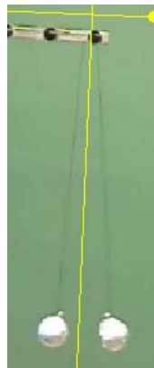
Figure 5: Still picture of charged pith balls in LoggerPro .
