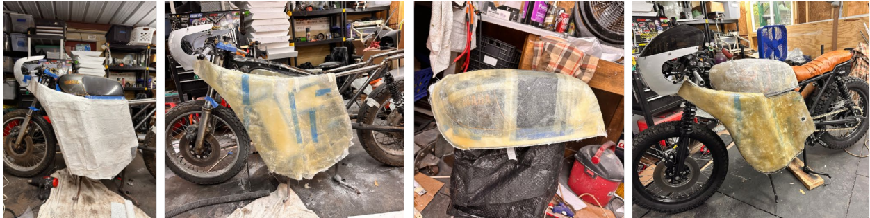
Appendix 8. Fairing and tank construction.
