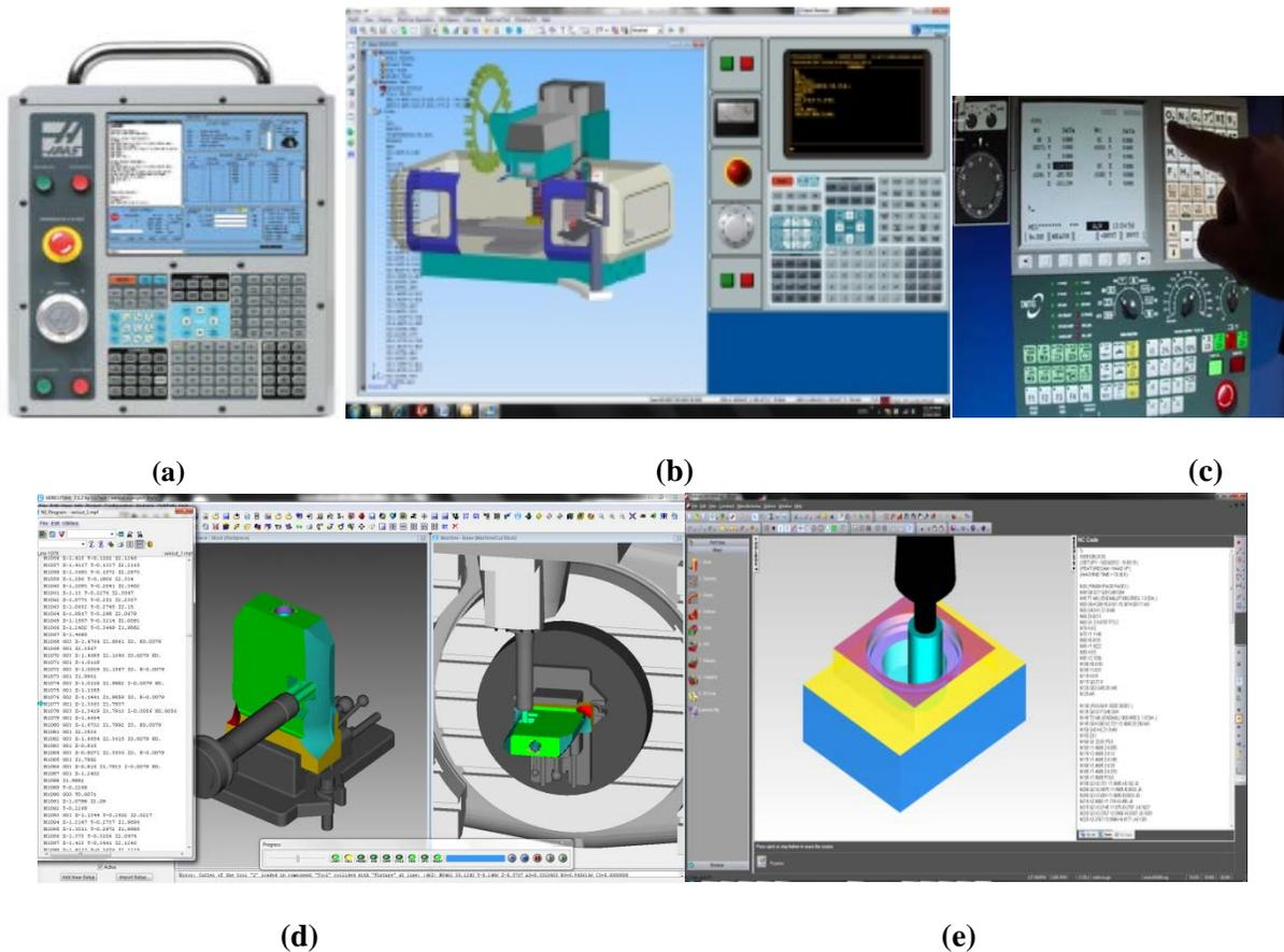
**Figure 4.** (a) HAAS dual system control simulator hardware. (b) Swansoft CNC simulation software showing machine control panel simulation for HAAS control. (c) Swansoft CNC simulation software showing machine control panel simulation on a tablet pc for Fanuc control. (d) VERICUT CNC machining and program verification software (e) FeatureCAM part program generation.
