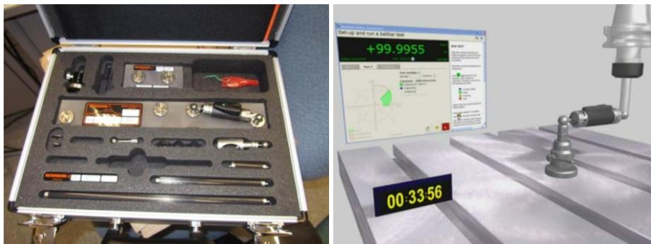
**Figure 1** Renishaw QC20-W (Wireless) Ballbar System in its protective carrying case (left) and Ballbar application simulation software (right)
