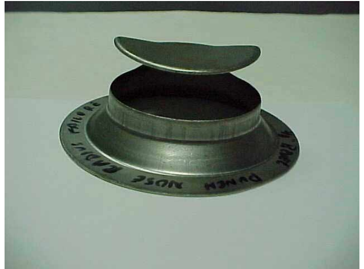
Punch nose radius failure
