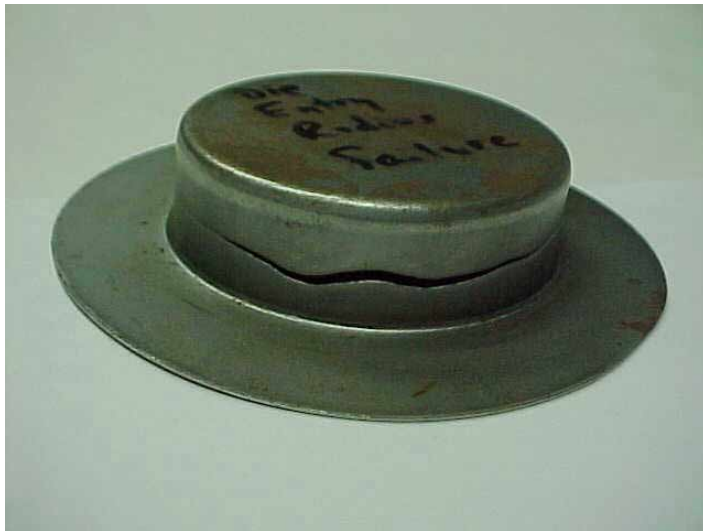
Die entry radius failure
