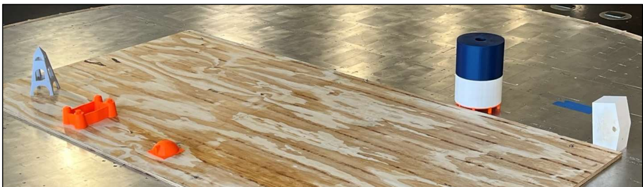
Fig. 6: Full-scale 3D printed models set up for slip (right) and for tip (left) are evaluated in the large wind tunnel.
