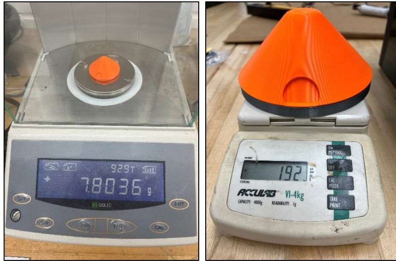
Fig. 3: Quarter- & full-scale 3D printed models were weighed for slip / tip calculations.
