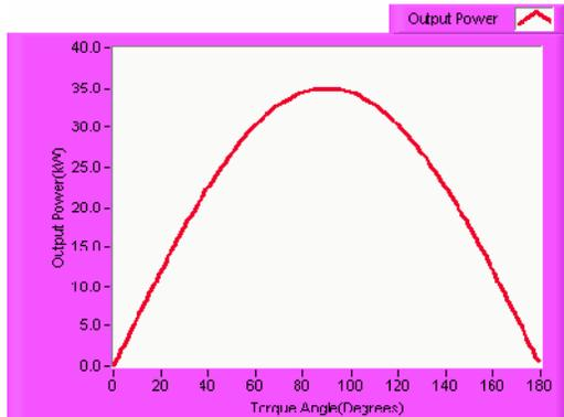
Figure 7: Graph generated in LabVIEW showing the variation of output power with the torque angle.
