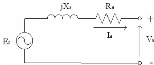
Figure 6: The per-phase equivalent circuit of the synchronous generator
