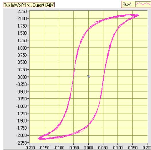
Figure 3: Hysteresis curve of a single-phase transformer.
