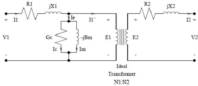
Figure 2: Equivalent circuit of a transformer
