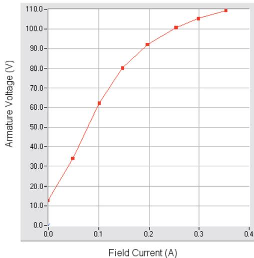
Figure 4: Saturation Curve of DC generator.
