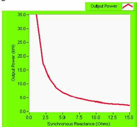
Figure 8: Graph generated in LabVIEW showing the variation of output power with the synchronous reactance.
