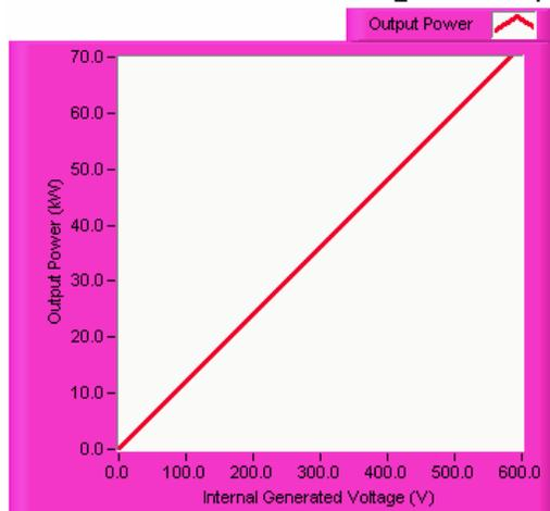
Figure 9: Graph generated in LabVIEW showing the variation of output power with the internal generated voltage
