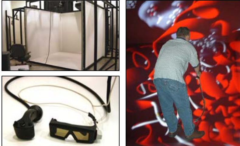
Figure 1. The CAVE, visualization equipment, and a user interacting with data inside the running CAVE.
