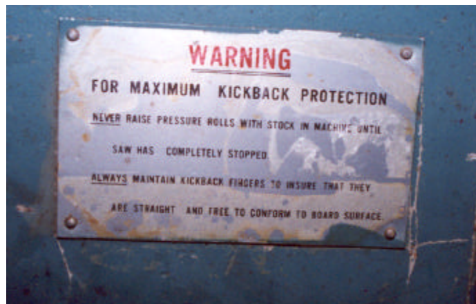
FIG. 7. WARNING Sign Which Uses Incorrect Colors and Format.
