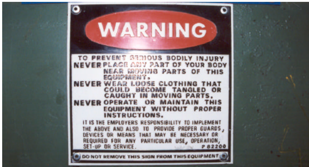
FIG. 5. WARNING Sign designated using Incorrect Color and Format.
