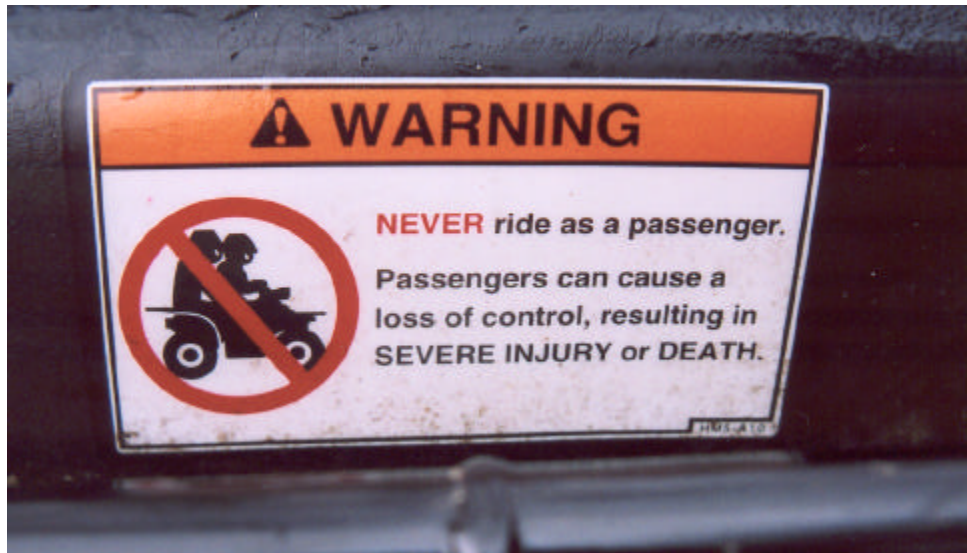
FIG. 4. WARNING Sign on ATV Containing all Proper Elements and Color.
