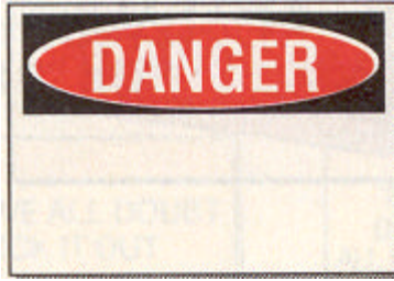
FIG. 1. Standardized Form for DANGER Signs Specified in ASA Z35.1-1941.
