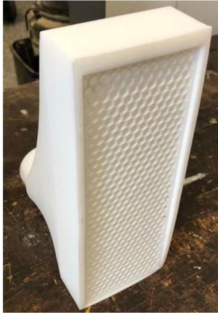
Figure 9: 3D printed diffuser with honeycomb insert
