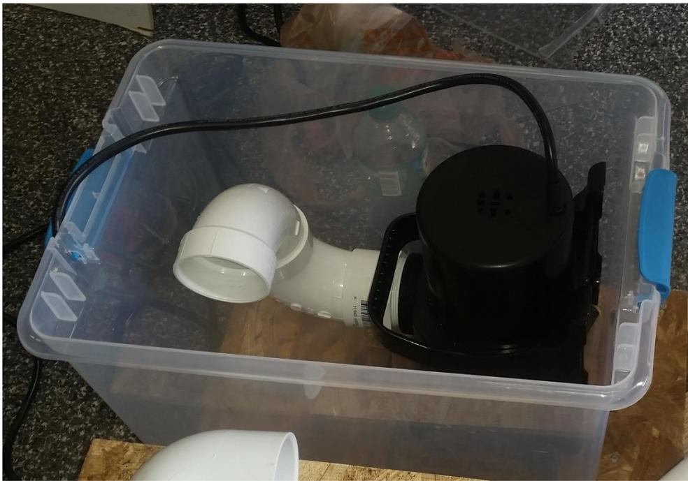
Figure 7: Submersible pump dry-fitted in reservoir
