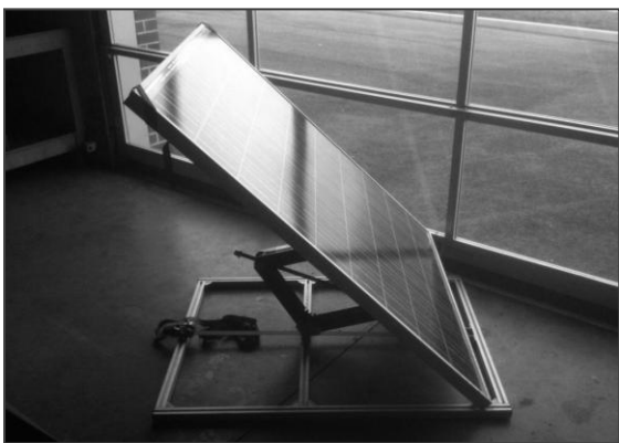
Figure 2: Solar Panel Mount Built by Undergraduate Rowan Students 7
