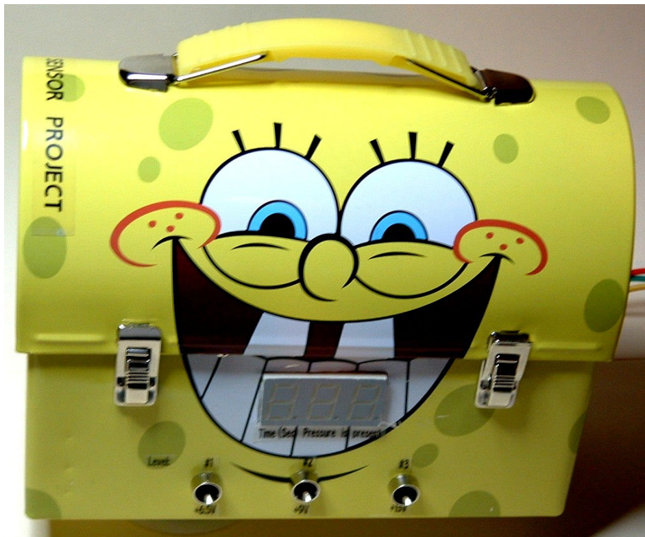
Figure 10 - Final Packaging Concept for the Pressure Sensor Project
