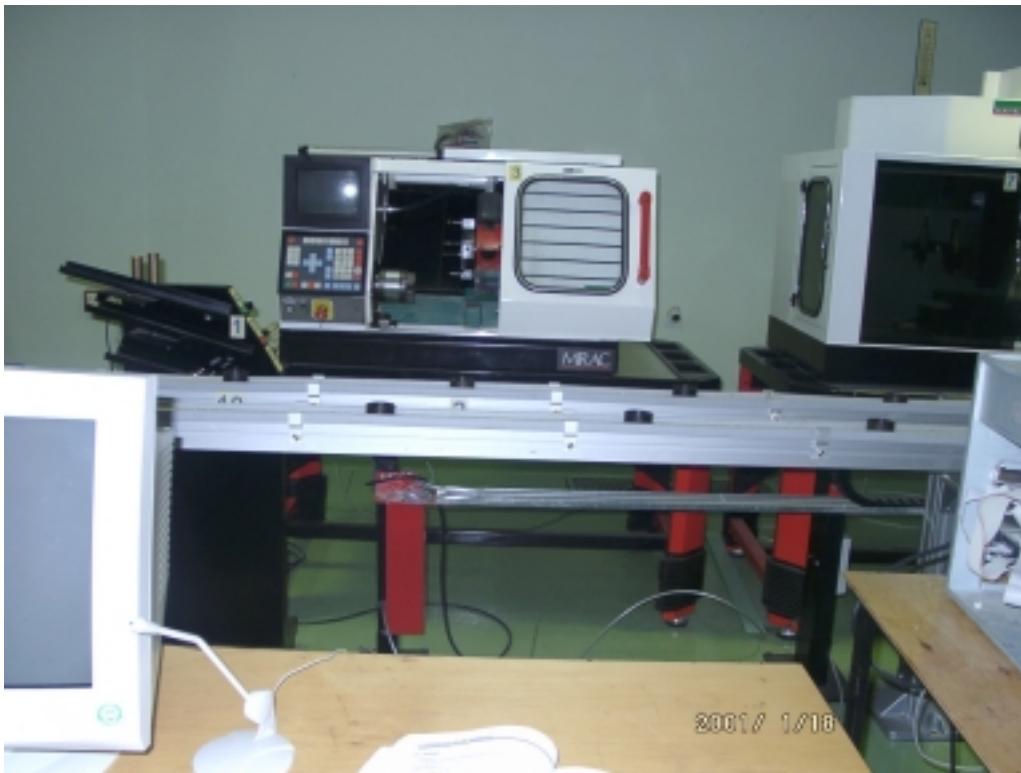
Figure 2 A closer look at the static buffer and CNC Turning machine
