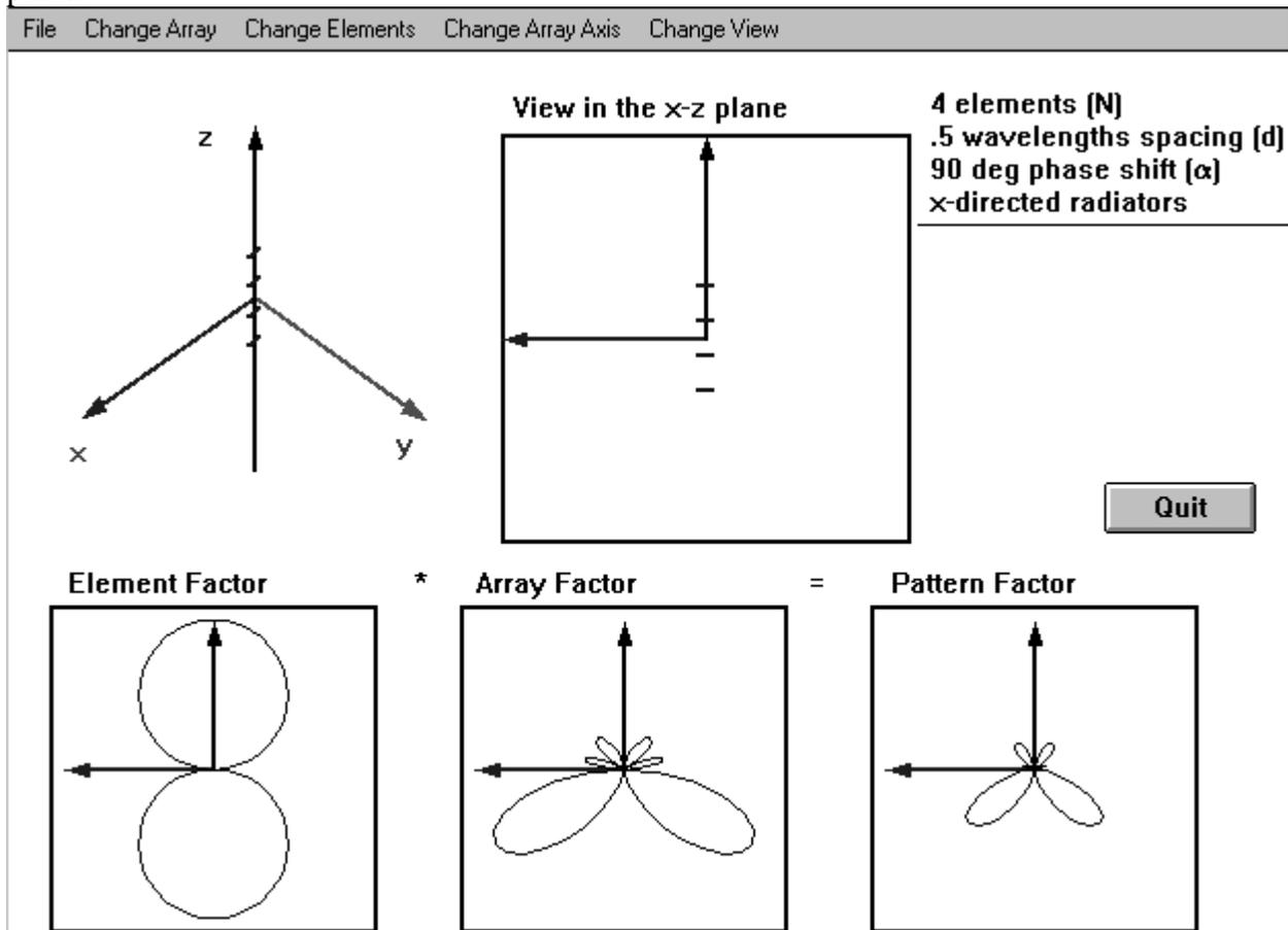
Figure 3. A four-element array of x-directed dipoles
