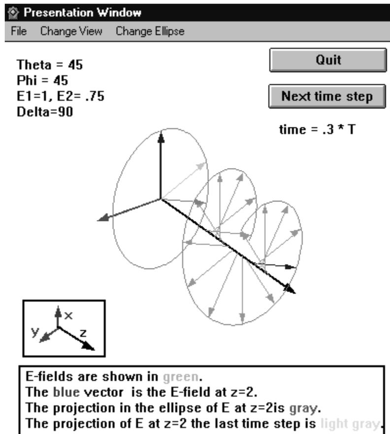
This module is an example of displaying a 3-D wireframe model in a two-dimensional screen window from the perspective of an arbitrarily placed observer. Conversion from the three-dimensional description of an object is performed using the set of subroutines shown in Figure 1 and excerpted in Table 1.
