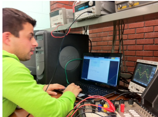
Figure 1. Students work in the software while engaged in physical lab activities. The student above sketches oscilloscope waves into the software (Figure 2) while recording phase shift and capacitive impedance on the oscilloscope (right). He draws VC, VR and V generator waves.
