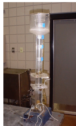
Fig. 2c. Two-phase Flow System
