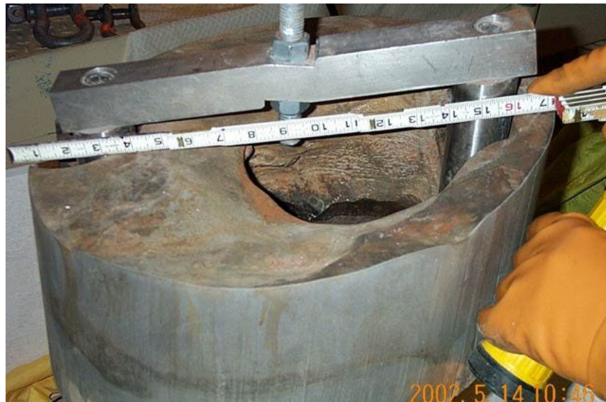
FIG. 4. Cutout from the reactor head with the football-sized cavity. See FIG. 1 for the location of the cavity in the reactor head. Photo: Blog.cleveland.com.
