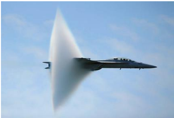
Figure 11: Pressure Cone: Beyond the Speed of Sound
