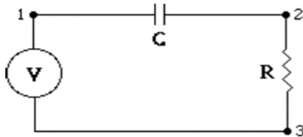
Figure 3. A series RC circuit
