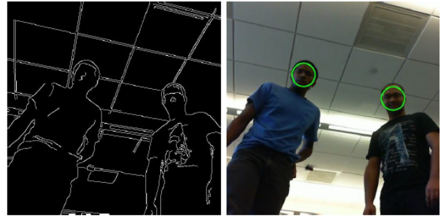
Fig 7. Experimental results for Computer Vision Evaluation on an image from WolfBot camera: Canny edge detection (left), and face detection using Haar cascades (right).
