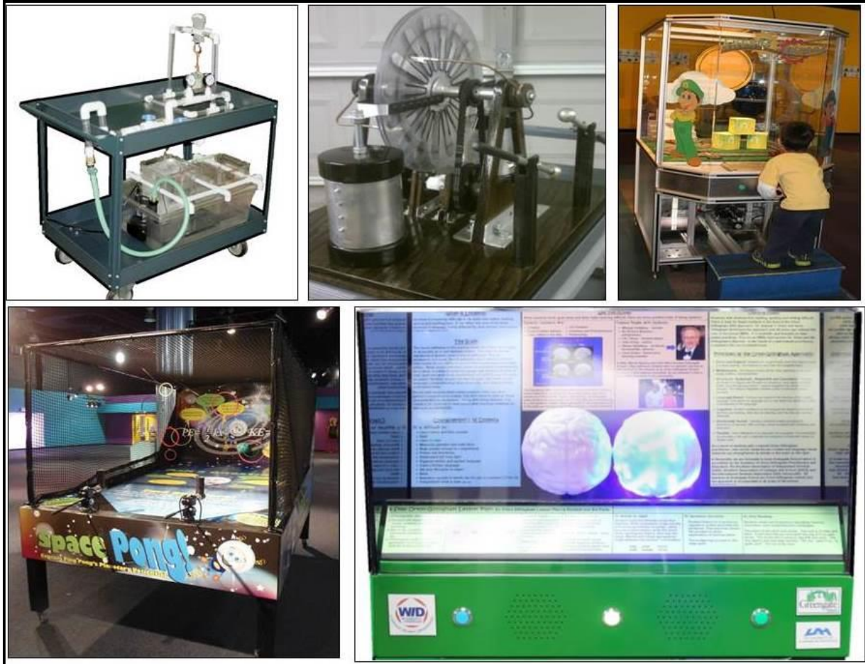
Figure 1. UAH/WID STEM tools, clockwise from top left: fluid flow circuit, Wimshurst machine, mechanical and solar energy race track, dyslexic brain display, “Space Pong”-potential and kinetic energy display ( photo credits: C. Carmen )
