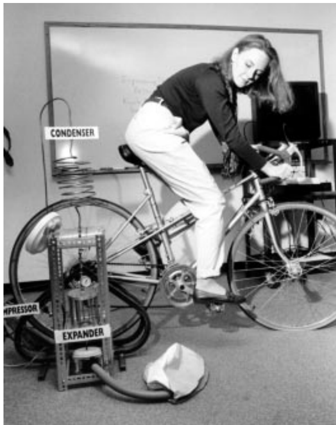
Fig. 1. Vicky Ryan, graduate of the University of Massachusetts Amherst Department of Mechanical and Industrial Engineering, demonstrates a bicycle-powered refrigerator for undergraduate students.
