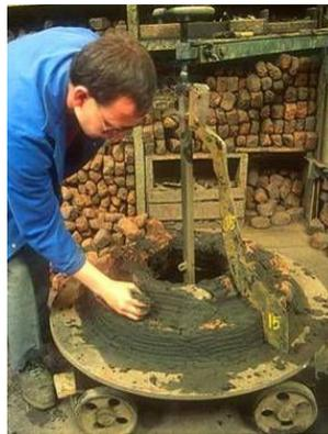
**Figure 12: A stickle is used in the process of creating a bell. A stickle smooths the inner and outer surface of a bell<sup>27</sup>.**
