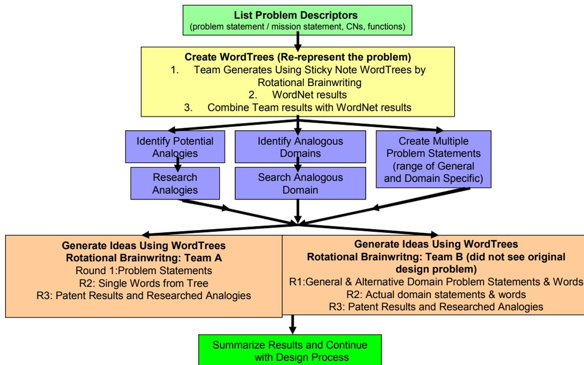
**Figure 2: Overview of the WordTree Design-by-Analogy Method.**
