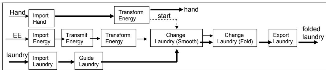
**Figure 4: Partial functional model for the laundry folding device.**
