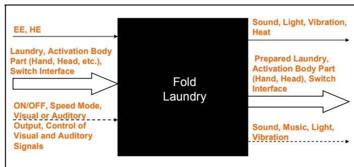
**Figure 5: Black box model for the laundry folding device.**
