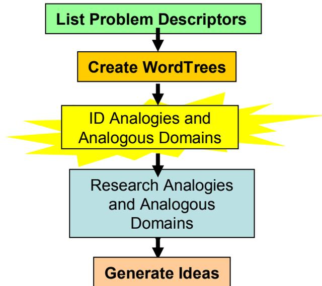
**Figure 9: Abbreviated WordTree Design-by-Analogy Method**
