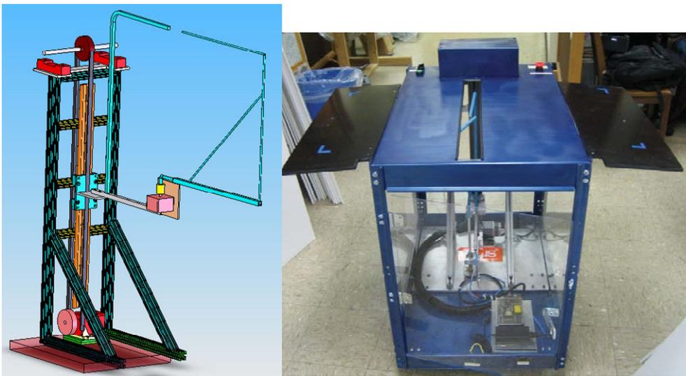
**Figure 11: Original team's award winning solution to the laundry folding problem. The image on the right shows the final solution and the left image is the internal mechanism. The towel or wash cloth is spread out on the top surface of the device. A bar rises in the center causing the item to fold in half. Half of the bar rotates around causing another half fold in the towel.**
