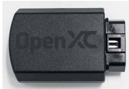
Figure 5. Ford Reference Vehicle Interface (VI) that enables Bluetooth communications with ODB-II.
