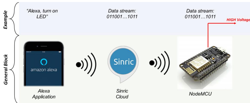
Figure 2. Workflow of information transmission from the smartphone to the NodeMCU.
