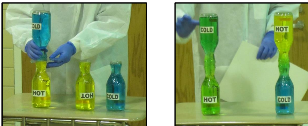
Figure 1. Allowing yellow colored hot water and blue colored cold water to mix.
