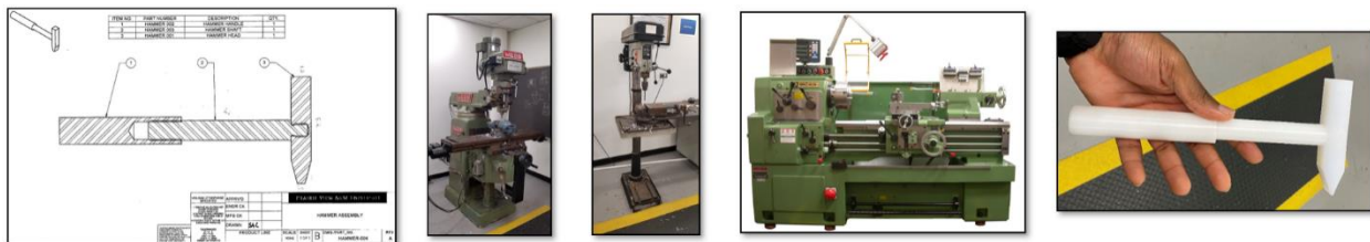
Figure 2. Students fabricated a predesigned plastic hammer using a manual mill, drill press, and lathe (center three images). A detailed procedure to create this hammer is designed in a virtual environment.
