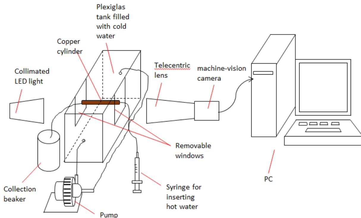
Fig.1. The schematic of the system, including the collimated beam of light, telecentric lens, machine-vision camera, tank with removable windows, copper tube, syringe, collection beaker, pump and the computer.
