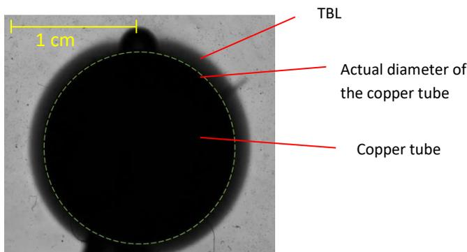
Fig. 2. Image from the video during the first few seconds following the start of hot water flow through the cylinder showing the diffusive growth of the boundary layer before buoyant convection became significant.
