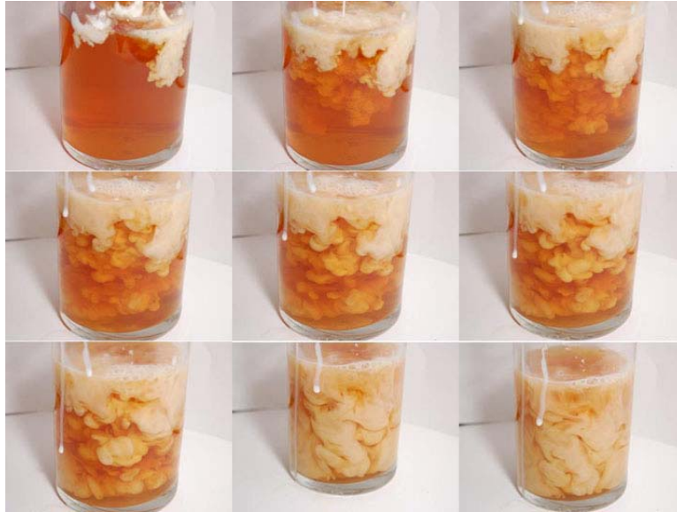
Figure 1. Example of student work: sequence of photographs by Kelly Rodriguez illustrating negative buoyancy of cold milk in hot tea.
