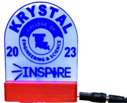
Figure 4. Desk lamp soldered, wired, and assembled during the INSPIRE workshop.
